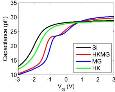
Figure 2: CV curves at 100 kHz for all samples at 25°C, they are not strongly frequency dependent
