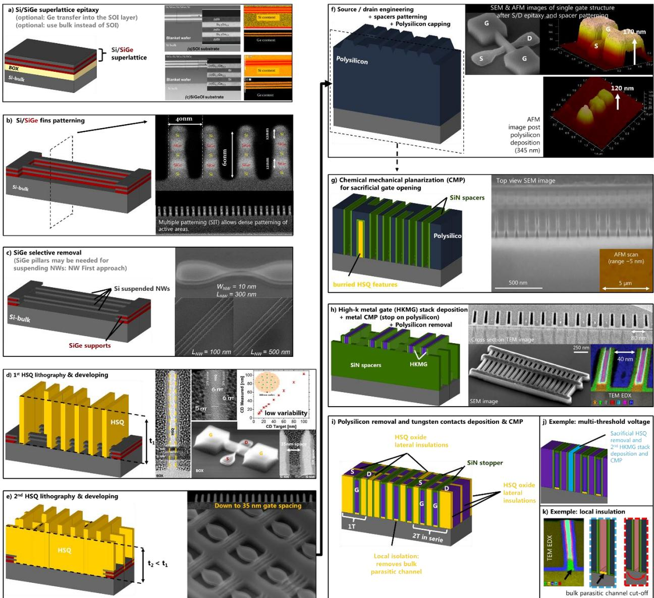
Figure 1. Gate last and NW first integration of SNWFETs: introduction to HSQ 3D lithography.
