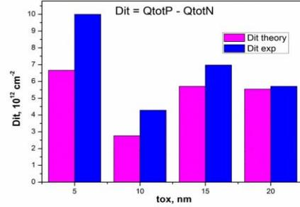
Figure 2. Integral density of surface traps in the  $\text{Al}_2\text{O}_3/\text{In}_{0.53}\text{Ga}_{0.47}\text{As}$  interface vs. thickness of  $\text{Al}_2\text{O}_3$ .
