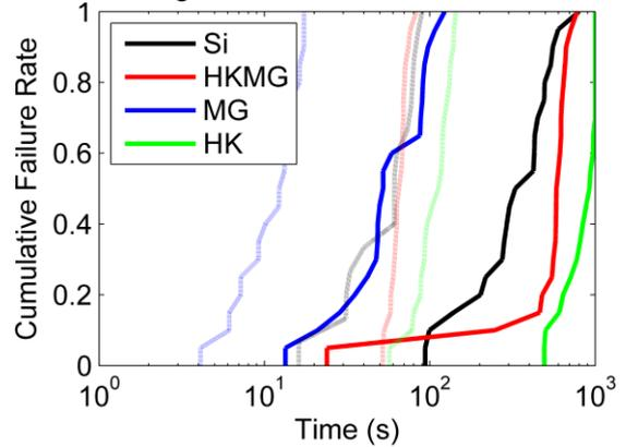
Figure 4: Cumulative failure rate at 125°C under gate stress of +17 V (solid lines) and +18.5 V (broken lines)
