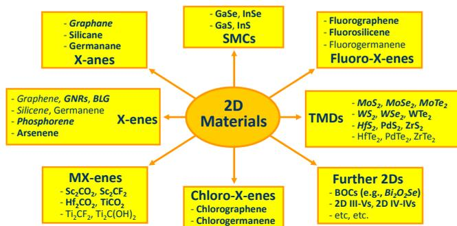
**Fig. 2.** Classes and representative examples of 2DMs. SMC: Semimetal chalcogenide. GNR: Graphene nanoribbon. BLG: Bilayer graphene. TMD: Transition metal dichalcogenide. BOC: Bismuth oxychalcogenide. Materials in bold letters: 2DMs with bandgap. Materials in italic letters: 2DMs already used in experimental FETs. After [10], updated.
