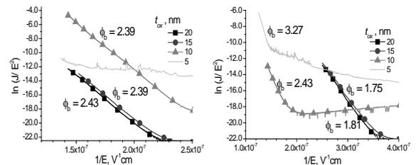
Figure 1. The FN plot for the the reverse bias branch ( $V_g < 0$ ) (a) and forward bias branch ( $V_g > 0$ ) (b) of  $J$ - $V$  characteristic of Pd/Al<sub>2</sub>O<sub>3</sub>/ $n$ -In<sub>0.53</sub>Ga<sub>0.47</sub>As/InP structure
