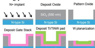
Figure 1: Schematic process flow for damascene capacitors
