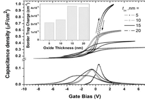
Figure 3. C-V characteristics of the  $\text{Pd}/\text{Al}_2\text{O}_3/\text{n-In}_{0.53}\text{Ga}_{0.47}\text{As}$  structures measured in forward and reverse directions and  $C_{\text{forward}} - C_{\text{reverse}}$  vs. gate voltage for different thickness of the gate dielectric. Inset: Border trap density as a function of  $\text{Al}_2\text{O}_3$  thickness
