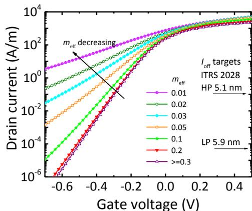
**Fig. 3.** Simulated transfer characteristics of 5-nm double-gate MOSFETs with channels showing different  $m_{\text{eff}}$ .
