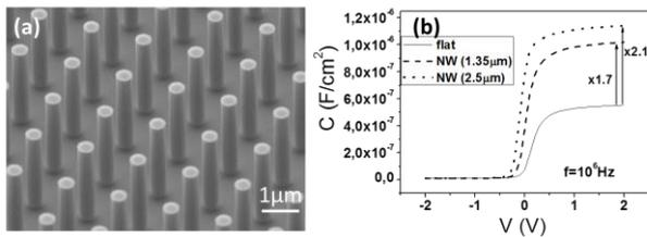
Figure 1. (a) SEM image at  $45^\circ$  angle of the sample with Si NWs of 2.5 $\mu\text{m}$  length and a 1.4 $\mu\text{m}$  pitch. (b) Capacitance density ( $C$ ) as a function of applied voltage ( $V$ ) for all three devices measured at a frequency of  $10^6$ Hz.
